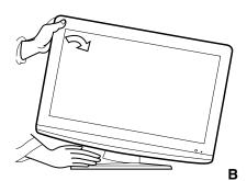
For wall mounting, the base must be removed. To disconnect the base/stand remove the two (2) screws from the back (see page 5).
